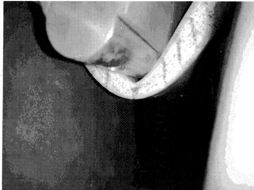
FIGURE 31: Final state of the sandwich 3 point bending test. Note the rigid fold in the top face causing the center to visibly separate from the loading roller.
