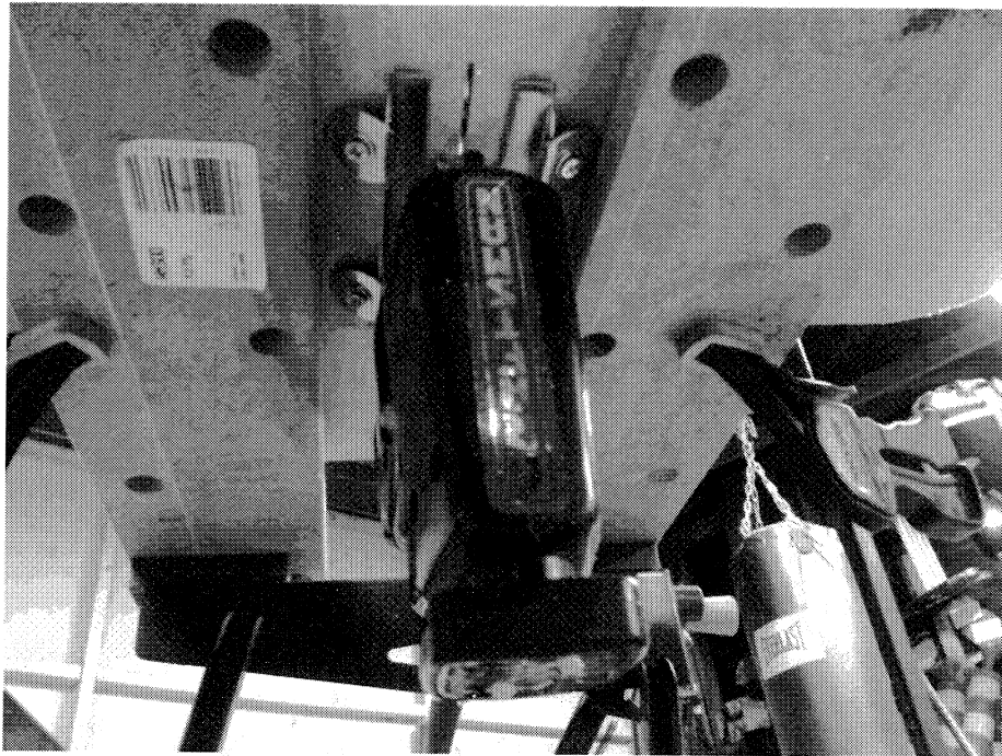
FIGURE 11: Underside view of the foam cutter showing how the jigsaw is mounted.
