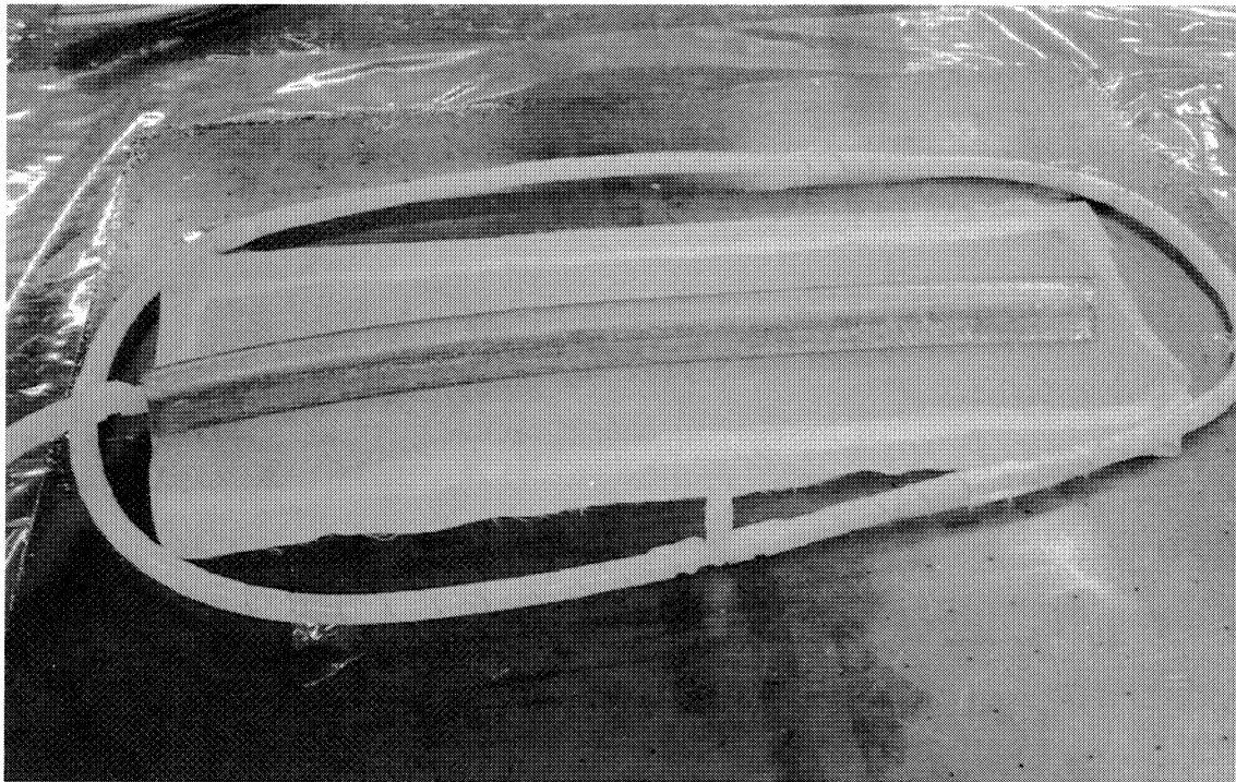
FIGURE 6: Pre-bagging layup of the hemp laminate. Showing the mesh (top layer), non-stick fabric (2 nd layer), steel plate, slotted hoses, and cable cover.
